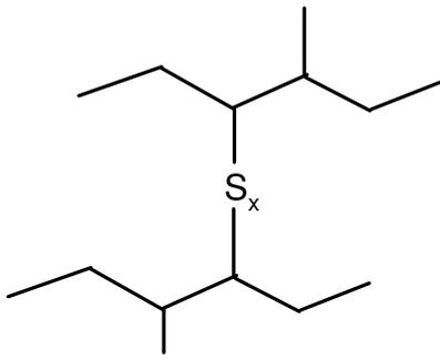
two adjacent Cis-polyisoprene chains, crosslinked with one (or more) atom(s) of sulfur
