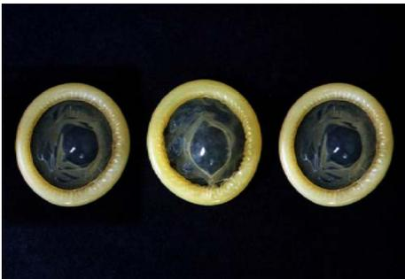
The condoms are now stored for up to 21 days to mature. This allows the material properties to stabilise before the condom progresses through to the next stages of the manufacturing process.
