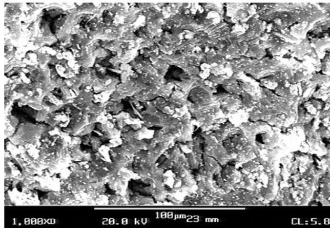
**Fig. 7:** Aluminium surface after application of 10% sodium hydroxide solution.
