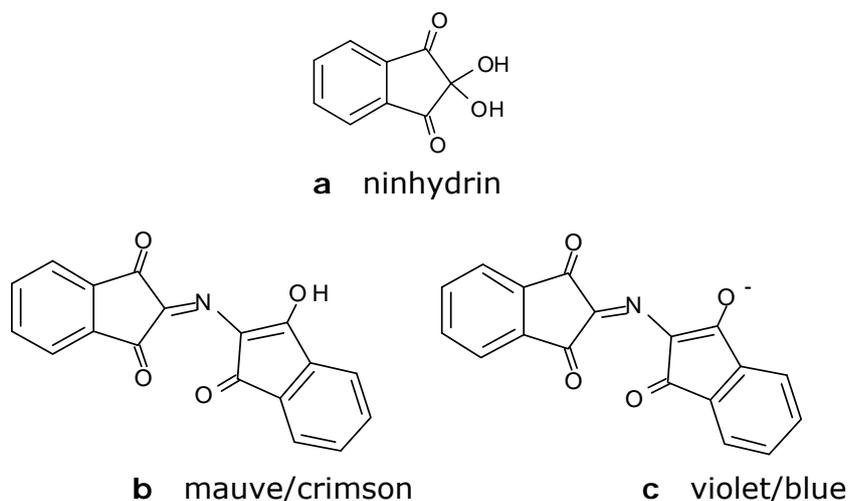
**Fig. 3:** structural formula of **a** ninhydrin and **b, c** the end products of the ninhydrin reaction (after [25, 27]).
