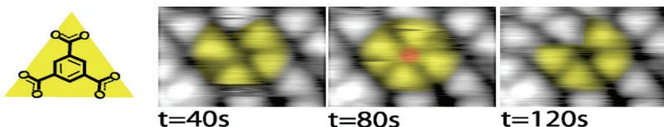
*Tma-molecules bond in a flat adsorption geometry at a copper surface are resolved as equilateral triangle in STM. The sequence of STM images reveals how the thermal motion of molecules at the surface proceeds. Following rational motions and displacements, a single Cu atom is captured whereupon a cloverleaf-shaped  $\text{Cu}(\text{tma})_4$  coordination compound evolves (second image for  $t=80$  s)*
